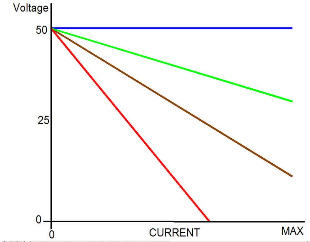
The above graph shows how the current control works. The voltage control is set at 50 volts. When set to the maximum (full clockwise), the voltage will stay at 50 volts (blue line) and is constant voltage. As the current control is rotated counterclockwise, the slope is increased. The red line is with the control fully clockwise.
