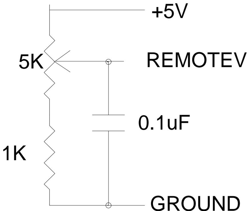
The potentiometer is the one in the footpedal. Use the current control to set the maximum current desired (full pedal setting.) Set the control board switches for remote contactor and voltage control.
