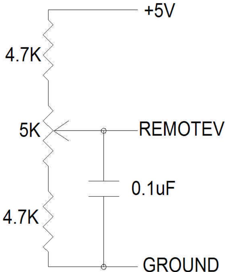
This will give a voltage range from 16.6 to 34.2 volts. If you do not plan on welding more than 100A or so, the upper resistor can be 10k. That will give about 16-25V out and an even finer control.
